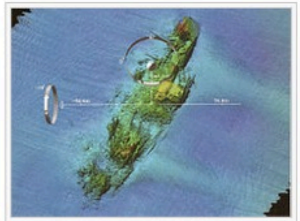
A multibeam image of the USS Susan B. Anthony (AP-72) shipwreck off coast of France.
