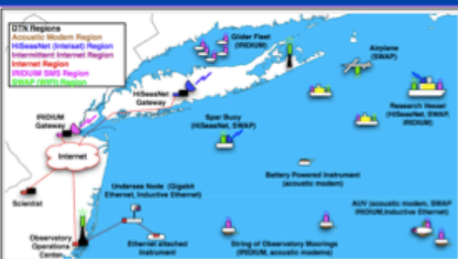
Figure 1. Hypothetical set of ships, AUVs, moorings, aircraft, gliders, and shore stations that make use of a variety of wireless communications devices and protocols. Platforms are grouped into regions based on common data communications needs and device usage.
