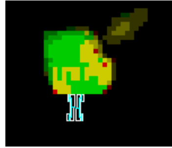
Fig. 3 Stereomap: the traversability mapper calculates the expected roll and pitch of the vehicle at each map grid cell in the sensor footprint using local least-squares plane-fitting on range data. The residual error of the plane fit is used as an estimate of the small-scale roughness of the terrain.
