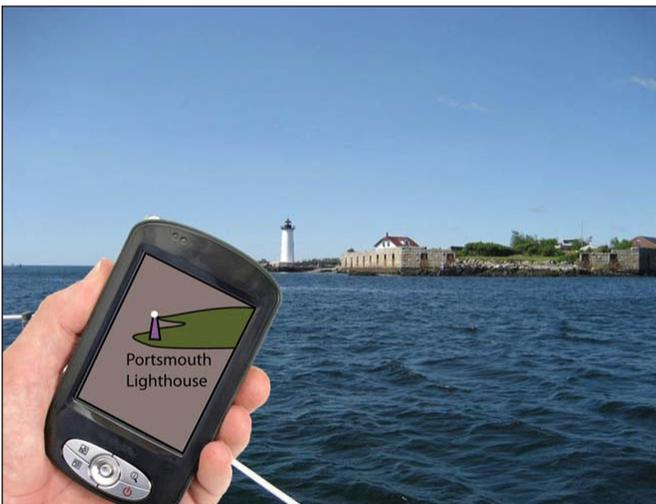
**Figure 39.** A mockup of a handheld spatially aware navigation aid. Note that precise registration is not needed to make the correspondence between chart objects and on-shore objects obvious.
