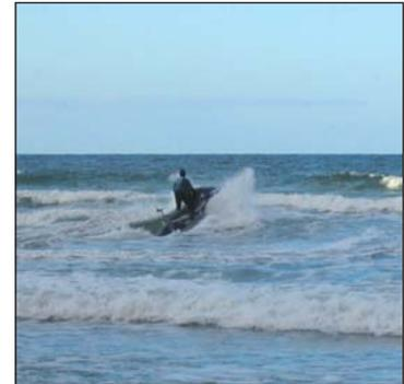
**Figure EX-4. CBASS surveying very shallow water through surf.**
