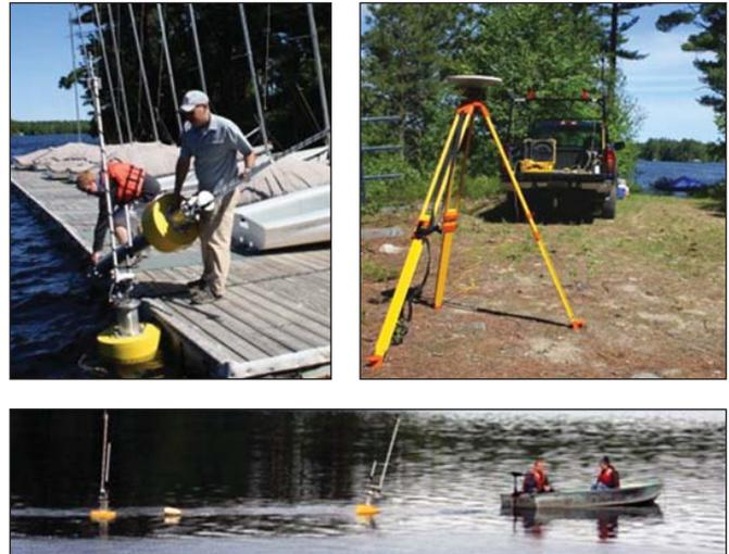
**Figure 50a.** Field trials at Mendums Pond. Upper left: Jon Hunt and Tom Weber deploying the buoys from the sailing dock. Upper right: the RTK base station used for broadcasting corrections to the buoys. Bottom: Jon Hunt and Michele Heller towing the buoys out for deployment.
