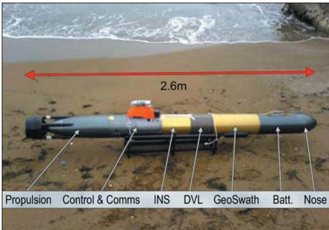
**Figure 45. GAVIA AUV with GeoSwath Phase Measuring Bathymetric Sonar.**
