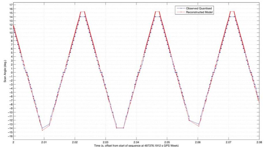
**Figure 20.** Example of observed, quantized, topographic LIDAR scan angles and reconstructed model angles using a Bayesian estimator. Effects of pattern irregularities, which appear to be active roll-stabilization of the LIDAR, cause complexities in the estimation that are not readily resolved using simpler estimators.
