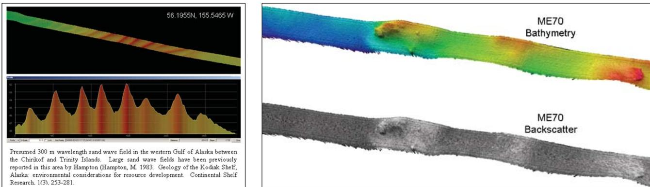
**Figure 17. Bathymetry and backscatter in the Shumagins (western Gulf of Alaska) showing rock outcroppings. Depths range from 80-120 m over the 6 km long transect. Data were collected using the ME70 multibeam echo-sounder, processed in custom MATLAB software, gridded and then plotted in Fledermaus. Note that the raw soundings processed in MATLAB have not been cleaned, giving an indication of the fidelity of the ME70 data.**
