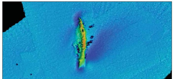
**Figure 18. Shipwreck of the *Andrea Doria* mapped in October 2009 by the NOAA FRV *HENRY BIGELOW* with the Simrad ME70 multi-beam sonar. Data were collected using a standard water column (non-bathymetric) mode.**
