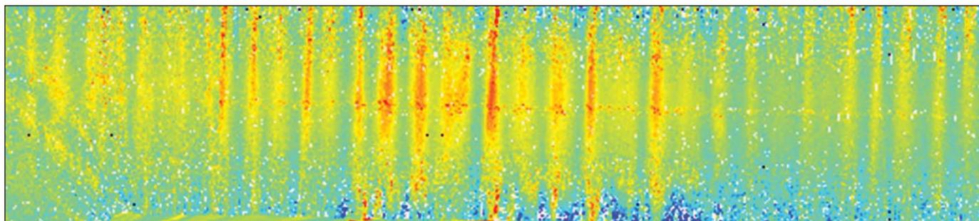
*Figure 47. Surface waves (swell) can induce pressure fluctuations in the depth sensor aboard the AUV, which is then imparted to the seafloor measurement shown here.*
