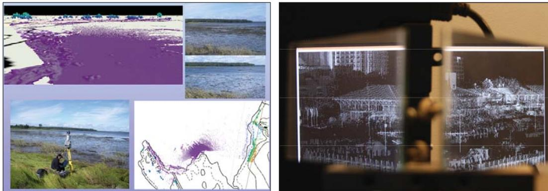
Figure 22. Left - Terrestrial laser scanning in Great Bay (September 10, 2009). Right - View of the Norfolk, VA vessel mounted LIDAR point cloud seen through the two mirrors of the stereoscope. The observer's brain will fuse the two images for stereo vision at the resolution of the human eye.
