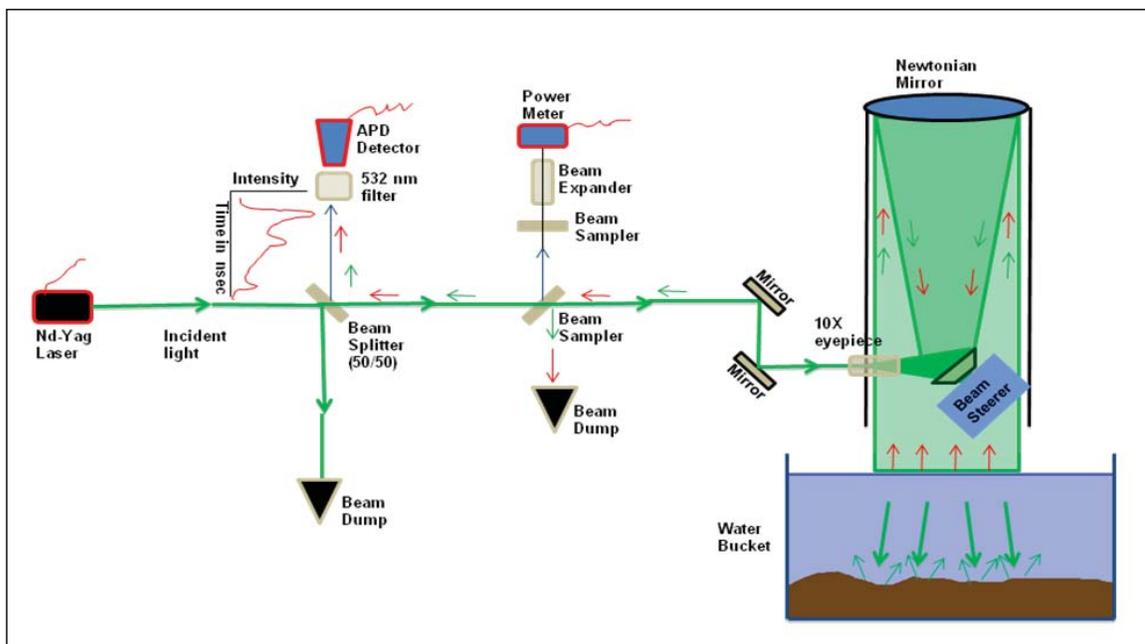
Figure 23. Schematic illustration of the bathymetric LIDAR simulator.
