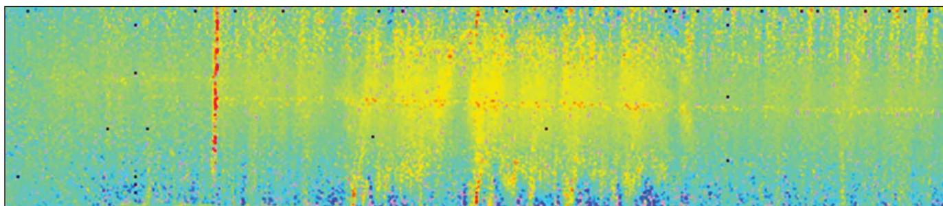
*Figure 48. Seafloor bathymetry in which the AUV's depth is taken from the inertial navigation sensor preventing the influence of short duration pressure fluctuations from surface waves.*
