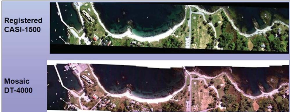
Figure 21. HSI co-registration: HSI co-registered (top) to a mosaic frame imagery (bottom).
