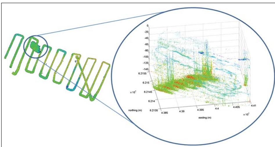
**Figure EX-9.** Seafloor backscatter (a proxy for bottom type), and the water column backscatter ( $S_v$ ) from the highlighted area collected with ME70 on *DYSON*. In the highlight, apparent bubble plumes appear light blue with a high vertical extent and narrow cross section. Rockfish appear aggregated in a ‘carpet’ around the base of the plumes (red and green).
