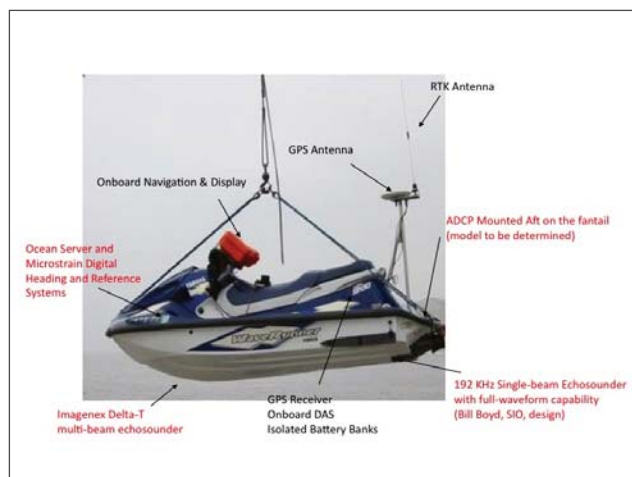
Figure 94. CBASS with principal components labeled. New components are indicated in red.
