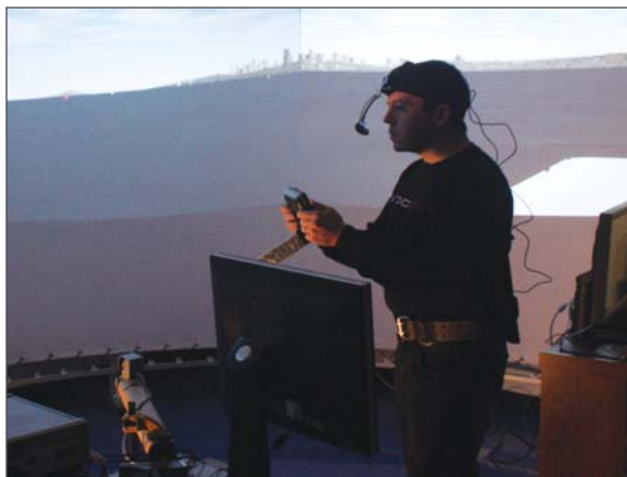
Figure 6. The virtual environment shipboard simulation developed to test alternative chart display techniques. Note eye-tracking apparatus on the participant's head.
