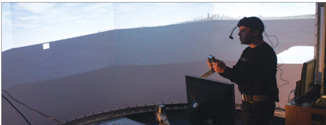
Figure 79. The virtual environment shipboard simulation developed to test alternative chart display techniques. Note the eye tracking apparatus on the participant's head.
