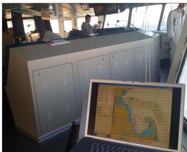
Figure 76. Aldebaran II on the bridge of an LNG carrier with Right Whale alerts on the ENC.
