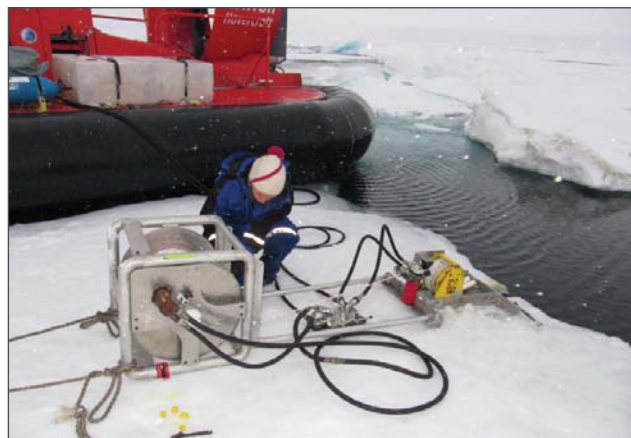
Figure 18. Hydrostatic corer being tested from Hovercraft Sabvabaa .
