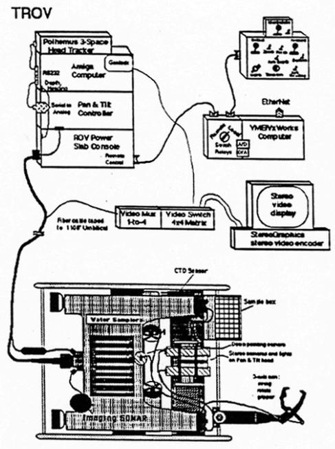
Figure 2: TROV components include: stereo pan and tilt cameras, downward point camera, 2 SONARs, manipulator arm with collection box, water column instruments, water sample collector.
