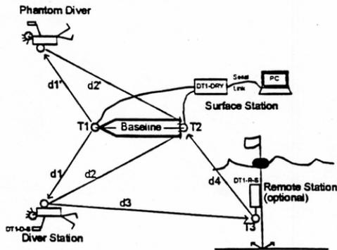
Figure 3. A typical DiveTracker system configuration used in Mono Lake.
