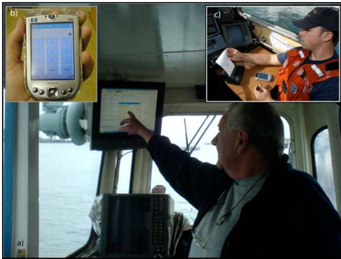
Figure 5. Simplified task-specific user interfaces can make using AIS much easier. a) The Thames River in England requires ferries to notify the local Vessel Traffic Service (VTS) with the number of passengers via AIS. b) With the right interface, an AIS application can be ported from fixed computer to a handheld. c) USCG Los Angeles station personnel using a PDA while working on a smaller patrol boat. Integrating AIS into these mobile devices can aid in incident response. Images from [33] and USCG.
