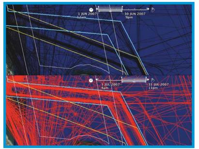
The top pane shows the vessel traffic pattern prior to the BTSS shift (June 1 to 10, 2007) and the bottom pane the vessel traffic pattern post-shift (July 1 to 31, 2007). The original BTSS is depicted in yellow and the new BTSS in blue. Monitoring demonstrated high compliance. Graphic courtesy of Dr. Kurt Schwehr.
