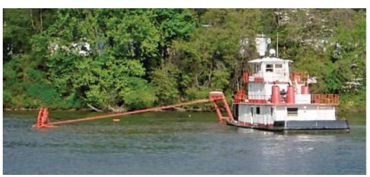
The UTV *Misty Dawn* the afternoon of April 18, 2010, shortly after the barge it had been pushing sank. The photo clearly portrays the minimal freeboard of the vessel and the two open doors along the port side of the vessel leading into the main engine and equipment spaces. All factors, combined with lack of watertight integrity, contributed significantly to the rapid progressive flooding of the main spaces and the subsequent sinking of the vessel later that night. U.S. Coast Guard photo.
