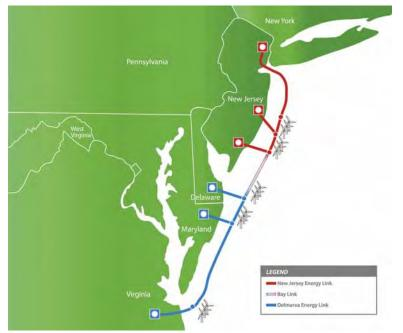
There will be six offshore platforms associated with the project, each capable of converting 1,000 megawatts of alternating current power (collected from the offshore turbines) to direct current power for delivery throughout the system.
