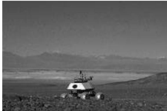
Figure: Nomad on a rocky field heading to the salar (ancient lake now dry). The association of ancient aqueous sedimentary deposits, channels, rocky and sandy fields, and volcanoes provided a good analog to planetary missions. The Andes in the background.
