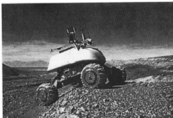
**Figure 3.** The Nomad rover crossing a channel. The ability of the rover to overcome difficult obstacles and challenging terrain allowed the science team to quickly reach distant science targets that proved to be critical for the overall understanding of the geological and biological history of the site.
