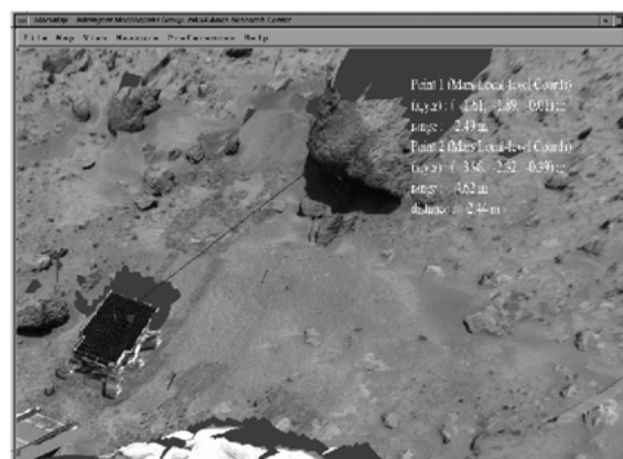
Figure 2. Measuring distance in Marsmap: from the robot Sojourner to the rock called Yogi.
