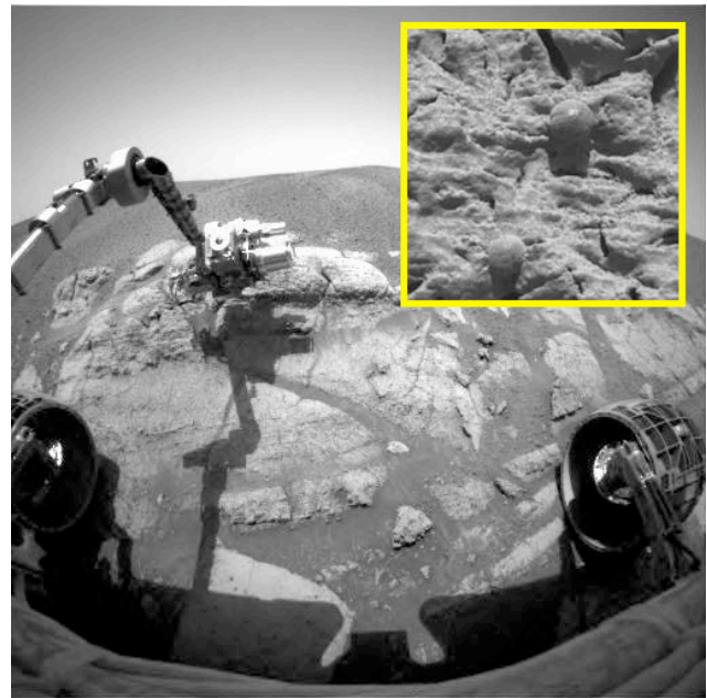
Figure 2b: The Rover Opportunity deployed its robotic arm also known as the Instrument Deployment Device on the El Capitan site. The inset image is from the Microscopic Imager (MI). Knowing the exact location of the MI image requires knowledge of the rover's kinematics state at the time of acquisition.
