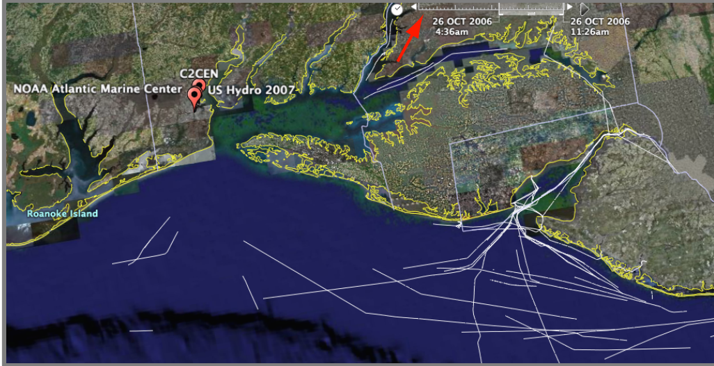
Figure 5: The marine National Automatic Identification System (N-AIS; [16]) provides position (white lines) and status information about vessel traffic in U.S. waters. N-AIS is still in development with coverage continually expanding as receivers are added to the network. The red arrow points to the time slider at the top of the figure that used to select a range of times. To the right of the time slider is a play button used to animate time data.
